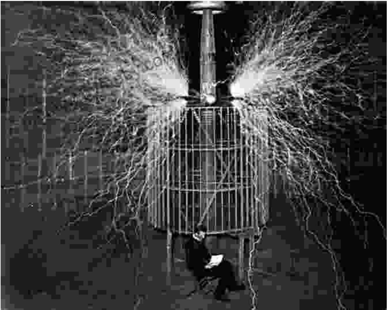
A Tesla coil generating electrical discharges.
